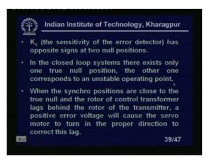
KS is the sensitivity of the error detector has an opposite signs at 2 null positions. It has opposite signs in 2 null position. In the closed loop systems there exists only 1 true null true position. And the other one corresponds to an unstable operating point on the system, right. Now, when the synchro positions are close to the true null and the rotor of the control transformer lags behind the rotor of the transmitter.
