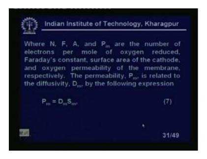
Where N, F, A and Pm are the number of electrons per mole of the oxygen reduced and Faraday's constant, it is FA is a Faraday's constant is a surface area of the cathode, which is very easy to calculate. Because it is a pi R square or pi D squire by 4 and the oxygen permeability Pm is the oxygen permeability of the membrane respectively right.
