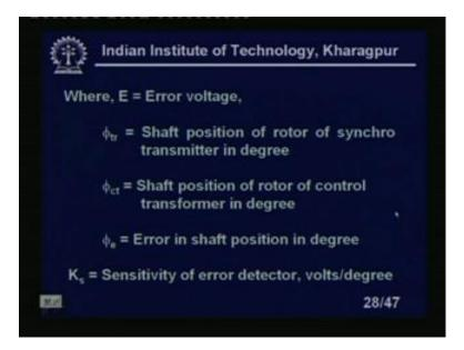
Where E is a error voltage phi tr is a shaft position of rotor, of synchro transmitter in degree, phi ct phi subscribes ct shaft position of the rotor of the control transformer in degree, phi e is the error in the shaft position in degree. And KS is the sensitivity of the error detector. It is in volts per degree.
