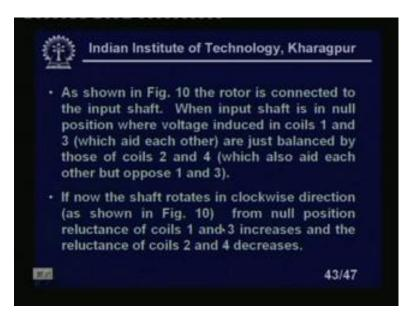
As shown in figure ten the rotor is connected to in the input shaft when the input shaft is in the null position, where the voltage induced in coils 1 and 3 which aid each other are just balanced by those of the coils 2 and 4 which also aid each other, but opposes 1 and 3 right. This is the balanced conditions; that means, the as I told you the voltage induced in the coils 1 and 3 which aid each other will exactly balanced by those of the coils 2 and 4
