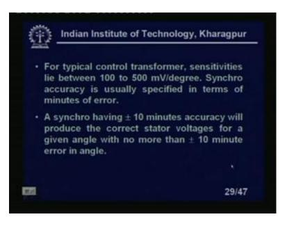
For typical control transformer, the sensitivities lies lie between 100 to 500 millivolt per degree. And synchro accuracy is usually specified in terms of the minutes of the error as you know 60 equal to 1 degree. A synchro having plus minus 10 of accuracy will
