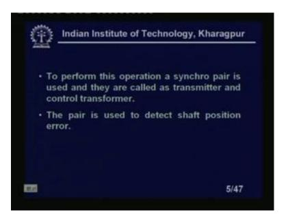
To perform this operation a synchro pair is used, and they are called transmitter and the controller transformer. Construction is almost same stator construction is almost same the rotor constructions are different, we will look at. The pair is used to detect shaft position later synchro pair as I told you, sometimes we are just calling it pair is used to detect the shaft position error.
