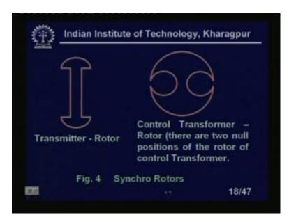
See this is the coil arrangement of the transmitter rotor, and this is the control transformer rotor. There are 2 null positions of the rotor of the control transformer. This is the synchro rotors constructions. You see this is dumbbell shaped whereas, this is cylindrical shape, why this is cylindrical shape? Dumbbell shapes already, I have defined. And why it is cylindrical shape? That we will define after few minutes.
