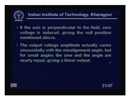
If the axis is perpendicular to the field 0 voltage is induced and giving the null position mentioned above. The output voltage amplitude actually varies sinusoidally with the misalignment angle, but for small angle the sine and the angle are nearly equal giving a linear output. How it is happened?
