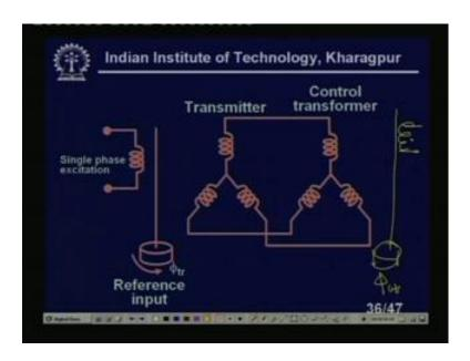
These we have shown, it is also spread up in the 2 this is a error synchro error detectors which I am going to show you, single phase excitations we have phi tr, we have phi ct. But it is spread over 2 slides, because this is a big diagram which cannot be accommodated on the single slide.
