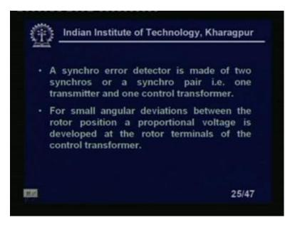
Now, synchro error detector is made of 2 synchros or a synchro pair or a synchro pair. that is 1 transmitter and 1 control transformer. For small angular deviations between the rotor position, a proportional voltage is developed at the rotor terminals of the control transformer right. That means, for small deviations it will find we have seen that it is the sinusoidal voltages. So, for small deviations near the vicinity of the null, we can use it as a linear sensor right.
