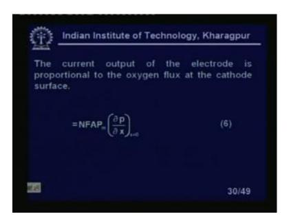
The current output of the electrode is propositional to the oxygen flux at the cathode surface. Now, NFA Pm will be equal to multiplied by partial derivative of P with respect to equal to 0; that means, at the cathode surface.
