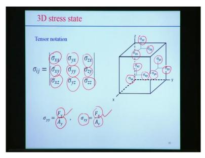
Now this time we try to focus on the 3 dimensional stress state. So far we know that the tensor notation of the stress analysis can be represented like that. Sigma XX, sigma XY sigma ZX, sigma yy and sigma zz. Now this stress notation, this stress tensor notation, we found out that there are 9 components of the stress, in case of 3 dimensional state, and out of that there are 3 normal stresses and 6 of the shear stress components.
