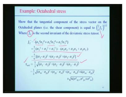
Now look into some problem then we need so that the tangential component of the stress vector on the octahedral plane, that means tangential component on the octahedral plan means the shear component here is equal to 2 third of J2 dot, where J2 dot is the second invariant of the deviatoric stress tensor. So here if we see that stress invariant is represented in terms of J2, so sometimes we use the in terms of I2 also and sometimes we use that stress invariant in terms of J also as well.
