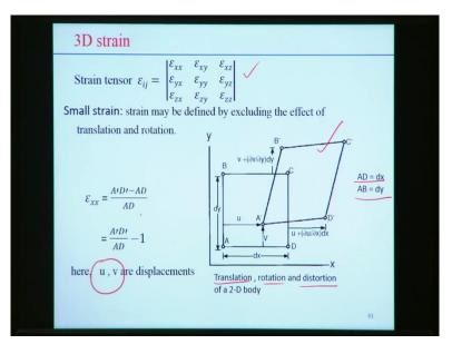
Now we will shift to the next topic that is called 3 dimensional strain and strictly focus on the small strain, so like stress tensor we can find out the strain tensor in the similar way, with respect to the axis x, y and z. But during the deformation actually it is subject to the translation, rotation as well as the distortion, specifically this figure indicates for the 2 dimensional body.
