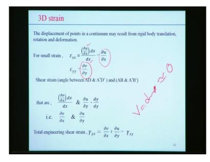
So corresponding to that, that is the difference and with respect to the initial level, so del u by del x actually represents the strain here. Similarly Epsilon yy that means y direction the normal strain can define del v by del y, so this is the partial derivative of displacement d with respect to x and y. Now we try to represent the strain, sheer strain basically in terms of the angular form, so in small distortion case the shear strain can be define, can be approximated, simply the angle.
