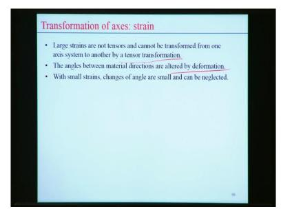
The angle between the material directions are altered by deformation that is also through because this large strain tensor we cannot transform using the simple transformation because in this case the angles between the material direction actually altered by the deformation, but with small strain change of angles can be neglected and we can use this transformation of the axis from one axis system to the another axis system, there is a small strain tensor exist.
