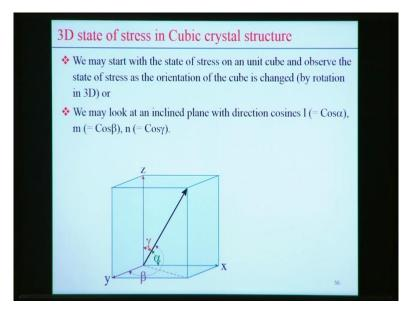
Now we come back to the what is the different type of stress state exists in case of cubic crystal structure, maybe we can start with the stress state on an unit cube and observe that the state of the orientation of the cube is changed by rotation in the 3D or we can take the view that will be a look in the inclined plane with direction cosine L, M and N.
