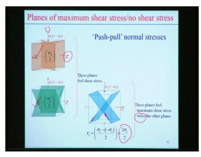
This is another case, for example push-pull normal stresses, that means tensile stress and another side is the compressive stress, with this situation specific plane which is subjected to but thus equal to minus, so here the two state of the stress but they are equally (())(57:18), but the direction is different, one is the tensile and another is the compressive. So in this case the maximum shear stress will be the by 2.
