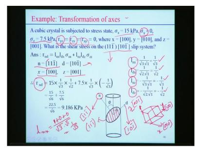
Now if you look into what example for that transformation of axis, you see that the example, we define the problem in such way that a cubic crystal is subjected to the stress state, sigma X equal to 15 kilopascal, for example sigma y equal to 0 and sigma z equal to 7.5 kilopascal so these are the stress state, normal stress to define at that x, y, z axis system but there is no shear stress acting on that, so we can simply say that tau yz equal to tau zx equal to tau xy equal to 0.
