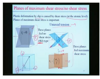
So let us investigate, physical investigate what are the different stress state actually exist in the cubic structure, so here is the most important, plastic deformation actually happens by the slip process at that atomic level, so within the cubic crystal structure it is more significant or important to know what is the maximum or what is the stress of the shear stress within the unit cell.
